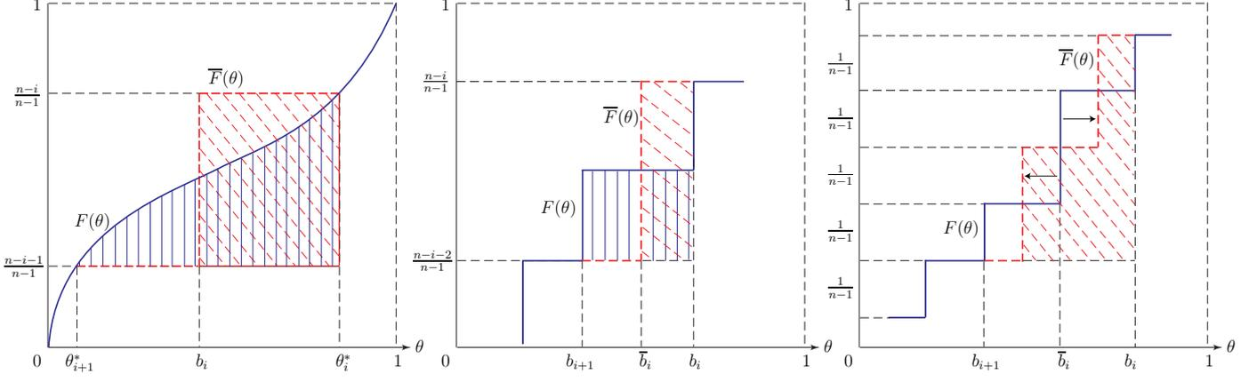
Figure 2: Step 1 (left): The area under the solid  $F(\theta)$  is replaced by the equally sized rectangle under the dashed  $\bar{F}(\theta)$ . Step 2 (centre): Combining two steps of the solid  $F(\theta)$  into a single step of equivalent ‘virtual’ weight. Right: Redistributing a double mass point in  $F(\theta)$  into its neighbours.
